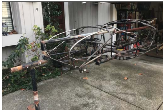
Rotisserie being used on a 1956 AC Ace chassis repair and restoration. The similarities with the 289 Cobra chassis are very evident. (January 2020)
