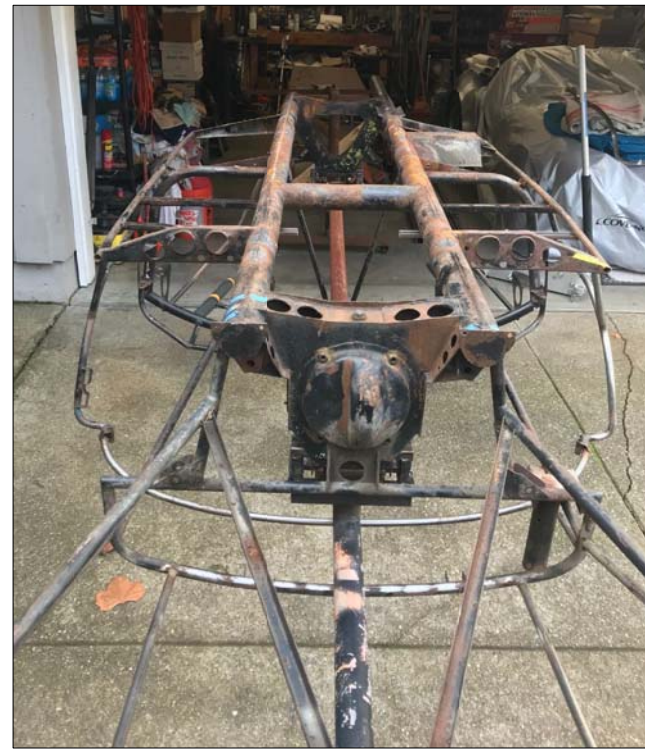
Rotisserie being used on a 1956 AC Ace chassis repair and restoration. The similarities with the 289 Cobra chassis are very evident. (January 2020)
