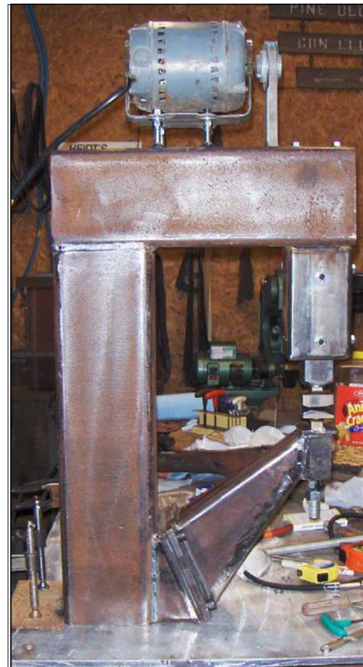
Photos of Reciprocating Shrinking machine under construction during the AllMetalShaping.com group build.
