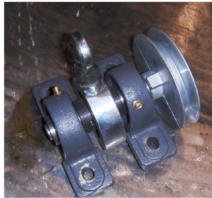
Pillow blocks, crankshaft and pulley assembly
