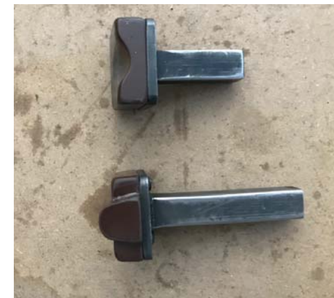
Nonmetallic thumbnail dies for aluminum shrinking (See Drawing number RS01 for details.)
