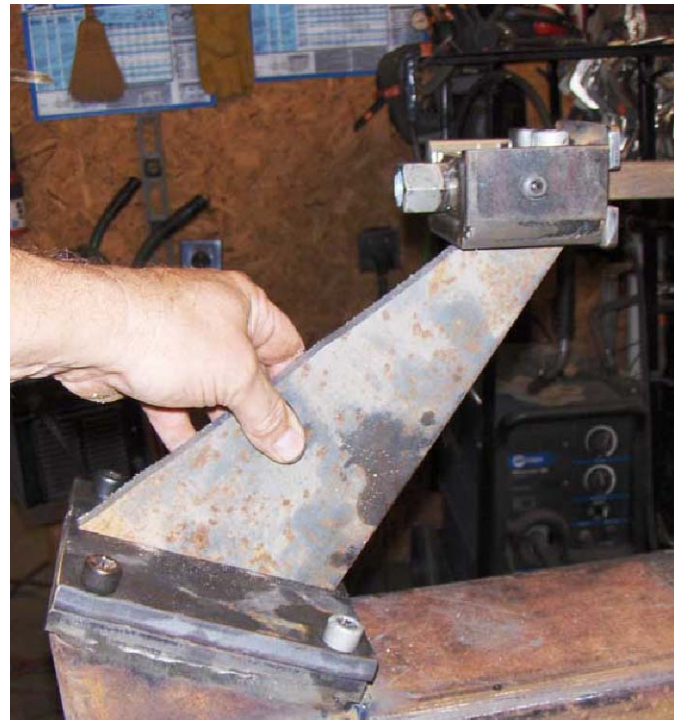
Lower tool arm and tool holder assembly
