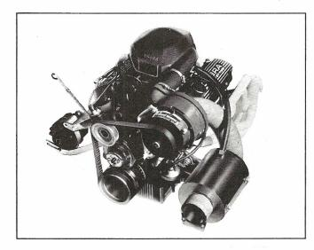
Supercharger kit contains centrifugal blower, carburetor enclosure, air cleaner / silencer, mounting brackets, pulleys, drive belts, gaskets, all necessary hardware, and complete instructions for installation.
